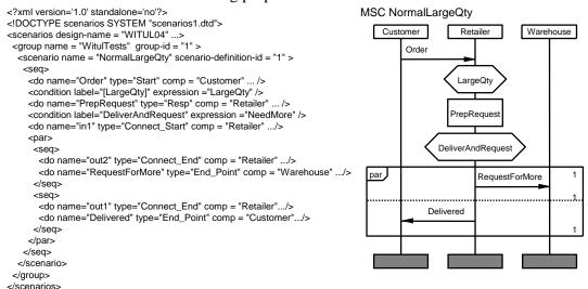
Fig. 4. Result of scenario definition NormalLargeQty, in XML and in MSC
