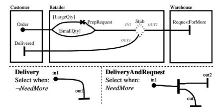
Fig. 3. UCM model of a simplified retail system: root map and plug-ins
