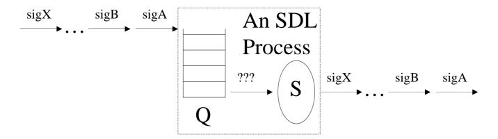
To build a queue which delays signals:
